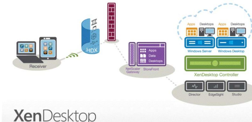
A typical XenDesktop environment consists of the following components:
