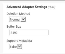
Deletion Method - This option controls how BLOBS are deleted. Audit: Files are renamed. Normal: Files are deleted. Shred: Files are securely deleted.
