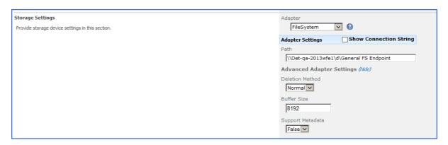
Click the *Show Connection String* checkbox to edit the connection string. Otherwise, fill in the connection fields shown for the adapter selected. Notice that the connection string parameters are name/value pairs separated by semi-colons.
