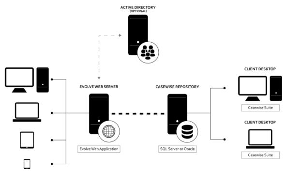
A typical installation of Evolve requires the following components:
