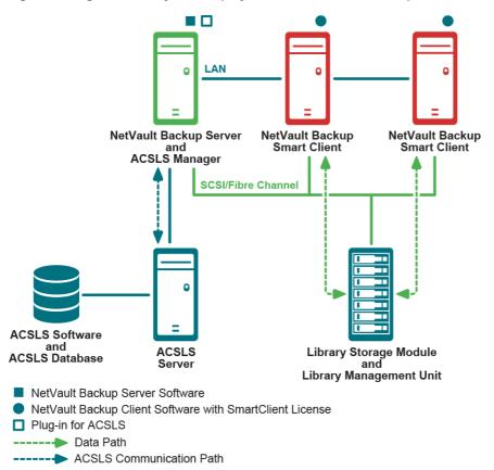
To control a single ACSLS System from the NetVault Backup Server but have the data flow directly from the NetVault Backup Clients to the Library Management Unit, perform the following steps:
