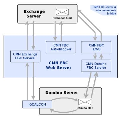
For technical reasons, QCalCon must be installed on the Domino server. The other four F/B Connector components may reside on a single server, as shown above.
