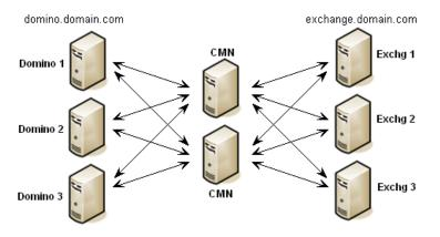
Multiple instances of the Mail Connector can be deployed for load balancing and to provide redundant mail paths.
