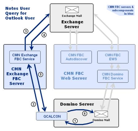
1 The Domino server sends a request for Sally's free/ busy information to Domino's internal queue, where it is picked up by the F/B Connector's QCalCon server task. (QCalCon resides on the Domino server and is configured to listen for Exchange calendar queries.)
