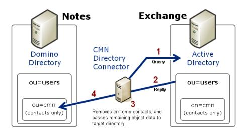
Each query–reply process as illustrated above is defined within the CMN Directory Connector as one *connector*. Two connectors defined for opposite directions, and run sequentially, together facilitate a bidirectional update. If you have multiple servers within either or both systems, the DC lets you define as many additional connectors as you need to facilitate updates among them.
