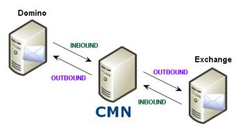
**Note:** The terms "Inbound" and "Outbound" as used here are relative to the Mail Connector itself, as shown in this illustration. An "Inbound" server is one *from* which CMN receives messages, and an "Outbound" server is one *to* which CMN relays messages.
