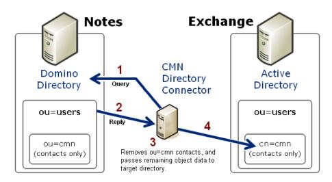
The Directory Connector then (3) filters (removes from the data) the objects that were in the source *ou=cmn* container. (The *ou=cmn* container is a reserved container created by the DC to hold contact objects copied from other connected directories. This filter eliminates the possibility of directory loops between connected systems.) CMN also maps the attributes of the remaining source objects to the corresponding contact attributes in the target.
