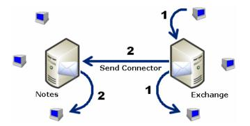
This diagram labels the Exchange smart host as the "Send Connector," which is the Exchange brand of smart host.
