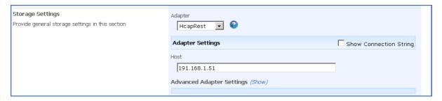
Click the *Show Connection String* checkbox to edit the connection string. Otherwise, fill in the connection fields shown for the adapter selected. Notice that the connection string parameters are name/value pairs separated by semi-colons.
