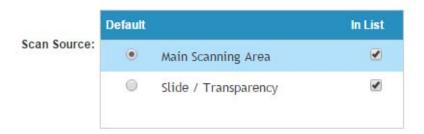
Scan source allows selection of Main Scanning Area or a more limited Slide/Transparency (used for X-ray and microscope scanning).
