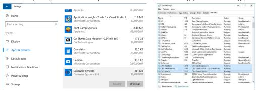
When uninstalling any version of Evolve from 4.0 upwards, it is also necessary to uninstall "Evolve Services" or "(CWS) Casewise Services" - the service that operates the Global Search.
