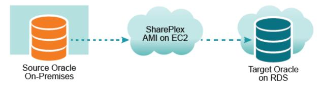
In this scenario, SharePlex runs as an Amazon Machine Image instance on the EC2 service. Capture connects to the source database through **TNS** and the Post process connects to the RDS database through **TNS**.
