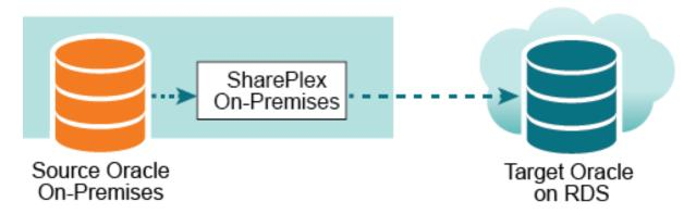
In this scenario, Capture, running on premises, connects to the source database through a **bequeath** connection and the Post process connects to the RDS database through **TNS**.
