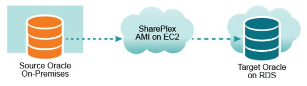
In this scenario, SharePlex runs as an Amazon Machine Image instance on the EC2 service. Capture connects to the source database through **TNS** and the Post process connects to the RDS database through **TNS**.
