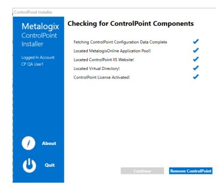
3 When the Component check has been completed successfully, click [Remove ControlPoint] to display the Remove ControlPoint dialog.
