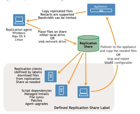
To create a Replication Share, identify one device at each remote location to act as a **Replication Device**. The appliance copies all the replication items to the Replication Device at the specified destination path. The replication process automatically restarts if it is stopped due to a network failure or replication schedule. If stopped, the replication process restarts at the point it was stopped.
