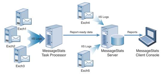
In this type of deployment, data from the remote Exchange servers is processed by the local task processor. Then the report-ready data is transferred to the MessageStats Server and stored in the database. This minimizes network traffic by eliminating the need to copy all the data from the remote servers.
