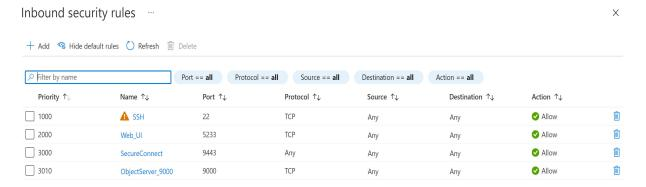
You can add rules as needed for corresponding functionality. For enabling multiple ports (like the case of RDA-NDMP), NSG allows port ranges and comma-separated lists of ports so that multiple ports can be enabled as part of one rule. However, the Marketplace offer configuration does not allow for ranges or comma-separated ports, so a Marketplace image's NSG template might mention each port number as a separate rule in such cases.
