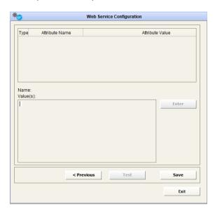
Pressing the button will store all the entered parameters for the web service adapter in the DT database.
