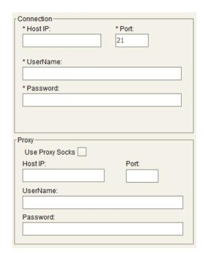
All the parameters in the Connection section are mandatory, including the FTP account to be used to access the specified directory; if a proxy is used then the user must complete the Proxy section parameters.
