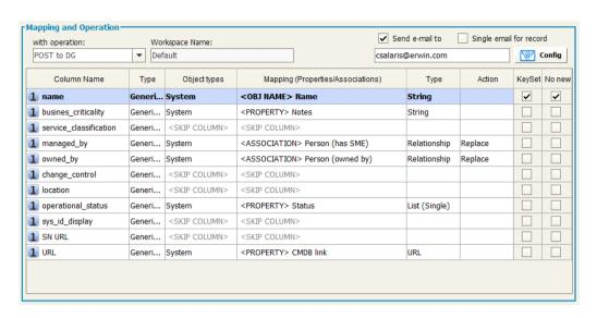
**Column type and format**: choose the type and format of the column of the source (String, numeric, boolean, date). This is important if user wants DT to perform a re-format operation on the target column data type.
