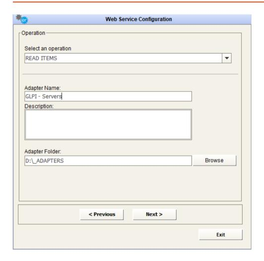
After selecting the desired operation, it is required to enter a name and a description for the adapter in the appropriate fields; the user must browse the file system for the adapter folder (used to save intermediate and result file for adapter execution).
