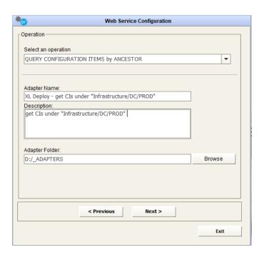
After selecting the desired operation, it is required to enter a name and a description for the adapter in the appropriate fields; the user must browse the file system for the adapter folder (used to save intermediate and result file for adapter execution).
