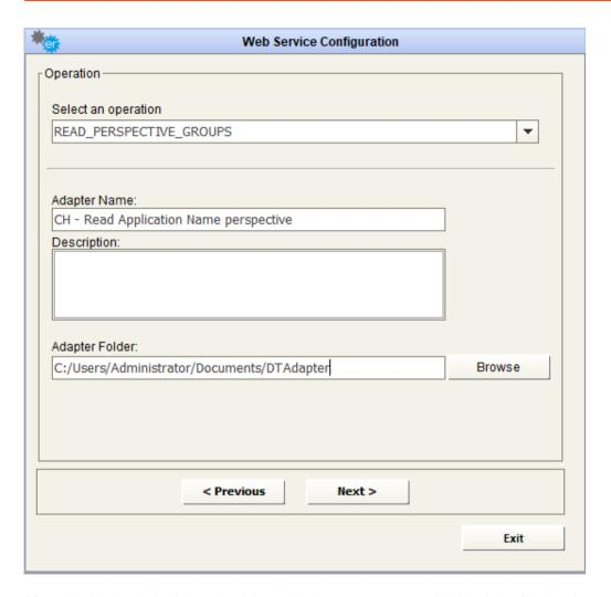
After selecting the desired operation, it is required to enter a name and a description for the adapter into the appropriate fields; the user must browse the file system for the adapter folder (used to save intermediate and result file for adapter execution).
