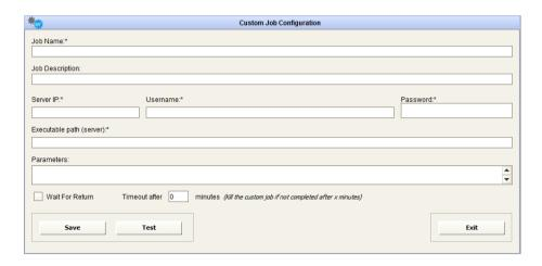
The user must provide the physical path, including the file name, of the given execution in the server, and the optional parameters required by the execution itself, enclosed by quotes if needed, as they would be written in a command line.
