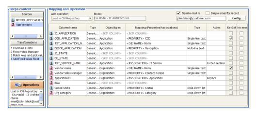
Note that the keyset for operation is set to "<Property> CIID" to manage the renaming of applications. The "Forced replace" option under 'Action' for "TXT\_SERVICE\_NAME" will make the association between "applications" and "IT services" be replaced even when associations are diagrammed.
