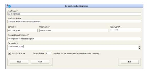
The option "Wait For Return" forces the process that launches the execution to be listening for the external process to end and wait for the exit code. In this case it's mandatory to define the timeout in minutes, to avoid DT hanging, if the executable does not exit in the given elapsed.
