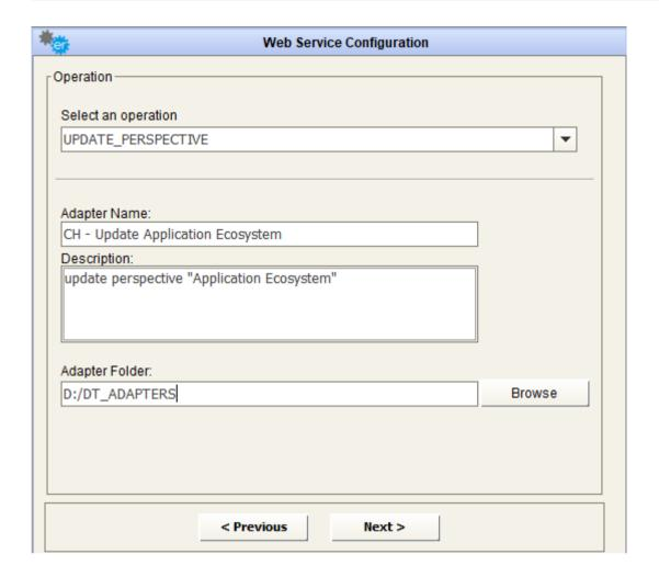
After selecting the desired operation, it is required to enter a name and a description for the adapter into the appropriate fields; the user must browse the file system for the adapter folder (used to save intermediate and result file for adapter execution).
