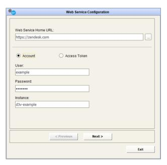
Click the button to proceed to the next step, and select the operation "Update Tickets". Enter a name and folder for the adapter. A description can also optionally be entered for the adapter.
