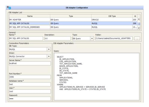
having the database type equal to "MySQL", server, port, database name, user, password and query producing the desired data (preview with the "Test" button):
