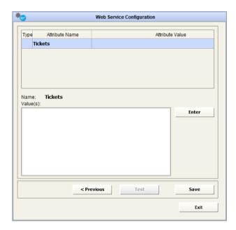
The adapter can now be used as a target endpoint when mapping data in a workflow. To select the adapter as a target, select "Web Service POST" as the operation and select your Zendesk adapter. A mapping table will appear, allowing the source fields to be mapped to relevant target fields for creating Zendesk tickets.
