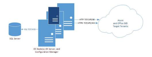
Figure 4. Ports used by Computer collections
