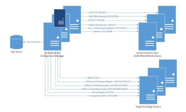
Figure 6. Ports used by File Storage Analysis collections
