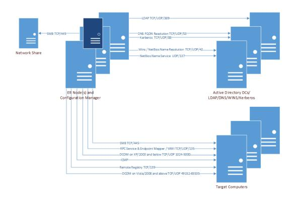
Figure 7. Ports used by NTFS collections
