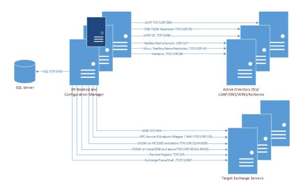
Figure 8. Ports used by File Storage Analysis collections
