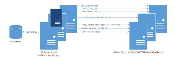
Figure 5. Ports used by Azure and Office 365 collections (Exchange Online, MS Teams, and OneDrive)
