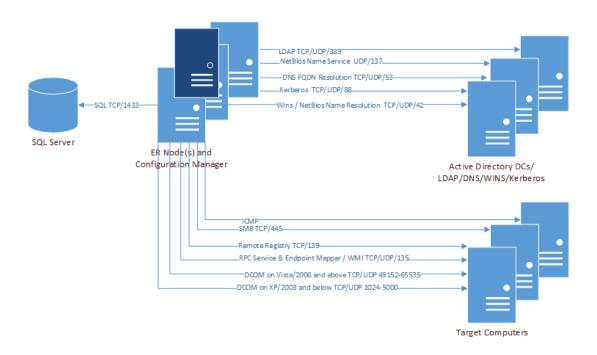
Figure 10. Ports used by Registry collections
