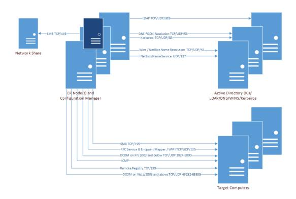
Figure 9. Ports used by NTFS collections
