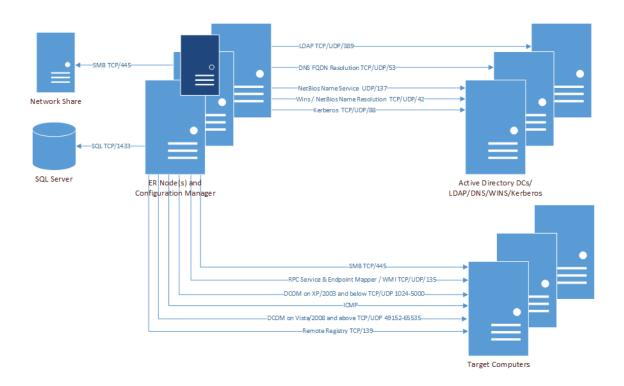
Figure 7. Ports used by Exchange collections
