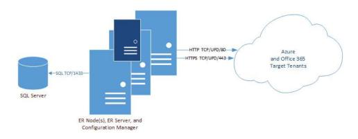
Figure 6. Ports used by Computer collections
