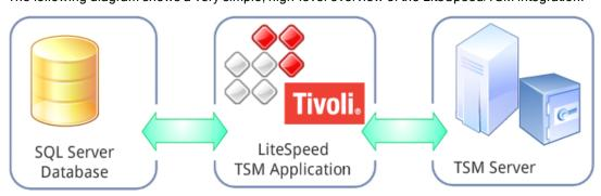
TSM backups conducted through LiteSpeed are transferred to and then stored in and/or managed by the Tivoli Storage Manager. The TSM handles the LiteSpeed backup file from then on, managing expiration date, storage location, etc. The functions of the TSM are not discussed here, please refer to the product documentation for further details.
