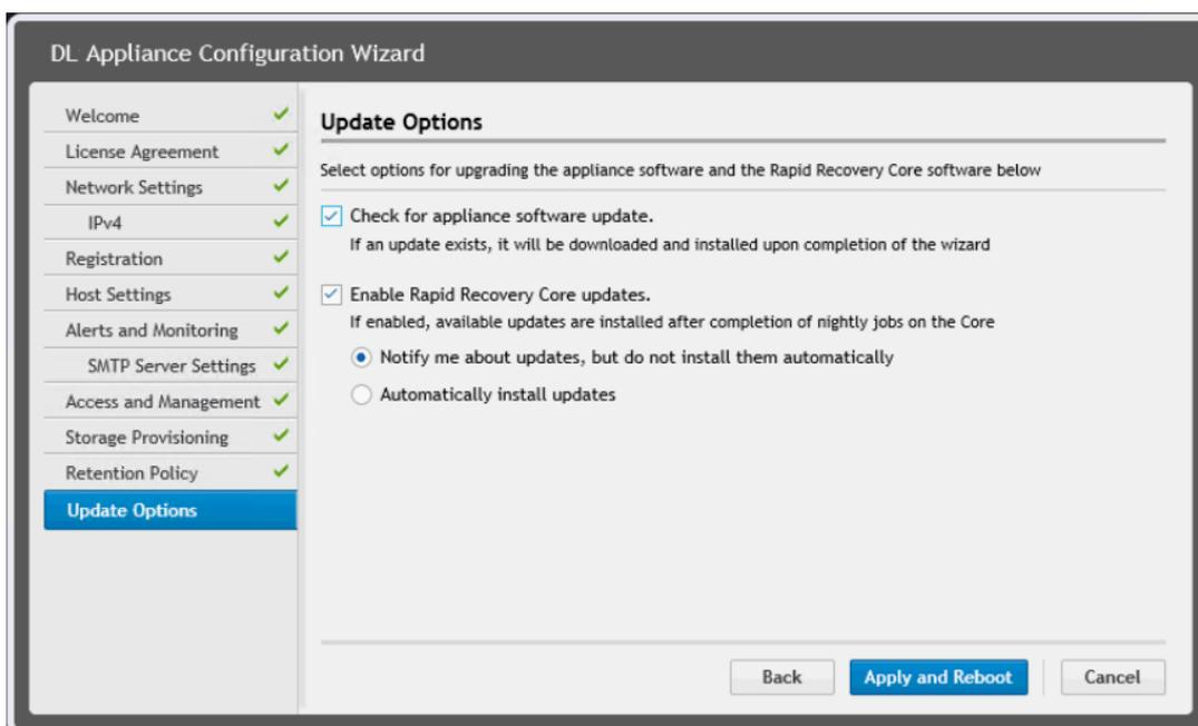
9. The appliance portion of the wizard is complete. The DL appliance will reboot if necessary, and proceed to the Machine Protection portion of the wizard.
