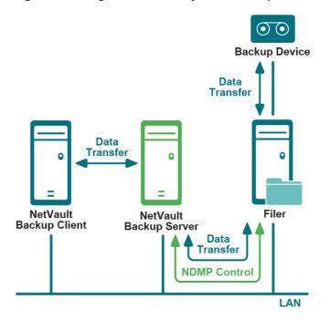
The heterogeneous three-way NDMP backup model is similar to the direct-attached model, but in this model the NetVault Backup machines on the network also use the filer-attached tape device for backups and restores.
