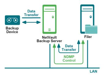
In the filer-to-server (filer-to-client) or remote backup model, the NetVault Backup Server instructs the filer to perform backups to tape devices attached to the server. The filer transfers the data and index information to the server using NDMP over the network.
