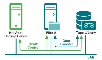
In this model, the NetVault Backup Server instructs the filer to perform backups to the NDMP-compliant networkattached storage device. The filer uses NDMP over the network to transfer the data to the storage device and backup index information to the NetVault Backup Server. The network-attached storage device can be shared by one or more filers, NetVault Backup Server and any number of NetVault Backup Clients.
