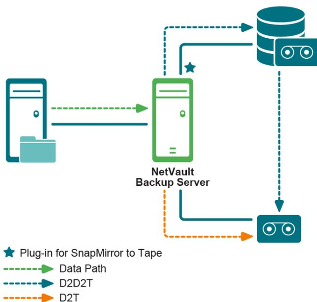
Figure 2. Deployment using filer-attached device
