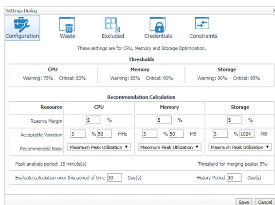
The Configuration tab provides recommended settings for CPU, memory, and storage optimization.
