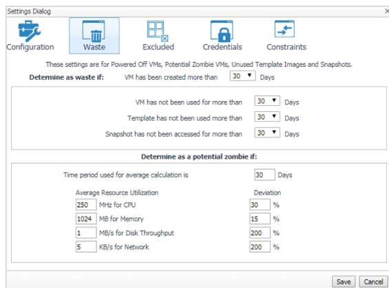
The Waste tab allows you to configure the settings for determining resources wasted in your environment. These include powered-off VMs, unused template images, snapshots, and potential zombie VMs:
