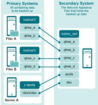
Before beginning a SnapVault configuration, you must also plan how many snapshots are required on a per volume basis; when they are to be updated; and how many of each are to be kept. Scheduling is decided upon based on the various values.
