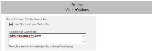
Default email addresses for system error and offline notification can be entered. Check the box to include the list of Default Notification Contacts specified on the General Settings page.
