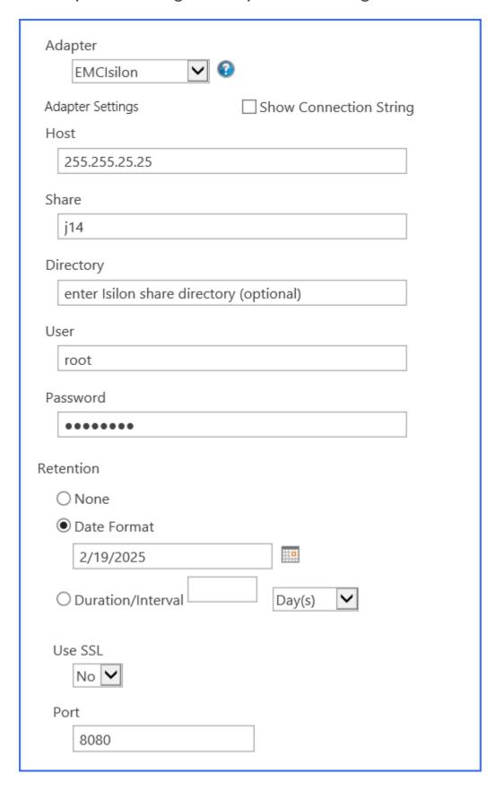
Click the *Show Connection String* checkbox to edit the connection string. Otherwise, fill in the connection fields shown for the adapter selected. Notice that the connection string parameters are name/value pairs separated by semi-colons when editing using the Show Connection String option.
