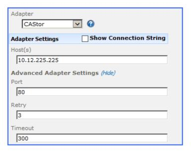
Click the *Show Connection String* checkbox to edit the connection string. Otherwise, fill in the connection fields shown for the adapter selected. Notice that the connection string parameters are name/value pairs separated by semi-colons.
