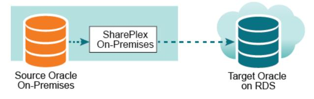
In this scenario, Capture, running on premises, connects to the source database through a **bequeath** connection and the Post process connects to the RDS database through **TNS**.
