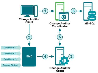
1 Using the client, users create an EMC Auditing template to configure the EMC file server (CIFS) location and select the agent to receive the EMC events.
