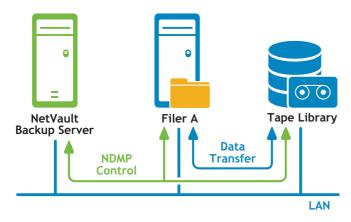
In this model, the NetVault Backup Server instructs the filer to perform backups to the NDMP-compliant network-attached storage device. The filer uses NDMP over the network to transfer the data to the storage device and backup index information to the NetVault Backup Server. The network-attached storage device can be shared by one or more filers, NetVault Backup Server and any number of NetVault Backup Clients.
