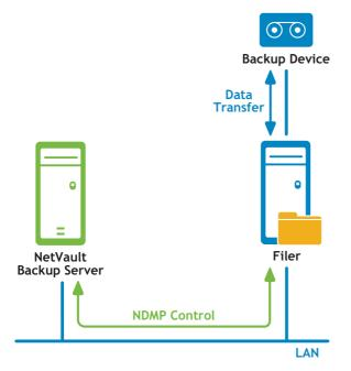
In the direct-attached or local backup model, the NetVault Backup Server instructs the filer to perform backups to the device directly attached to the filer (through Fibre Channel or SCSI). The filer transfers the backup index information to the server using NDMP over the network. During restores, the filer reads the data from the direct-attached device on server instruction. The actual data is not transmitted over the network during backup or restore, eliminating network congestion altogether.
