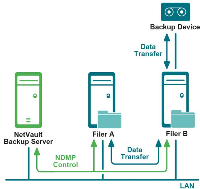
In the filer-to-filer or three-way backup model, the NetVault Backup Server instructs Filer A to perform backups to the tape device attached to Filer B. Filer A transfers the data and backup index information over the network. Filer B transfers the data directly to the device; it transfers the backup index information to the server using NDMP over the network. This model allows sharing of tape libraries among multiple filers.
