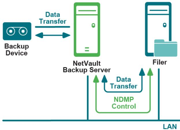
In the filer-to-server (filer-to-client) or remote backup model, the NetVault Backup Server instructs the filer to perform backups to tape devices attached to the server. The filer transfers the data and index information to the server using NDMP over the network.
