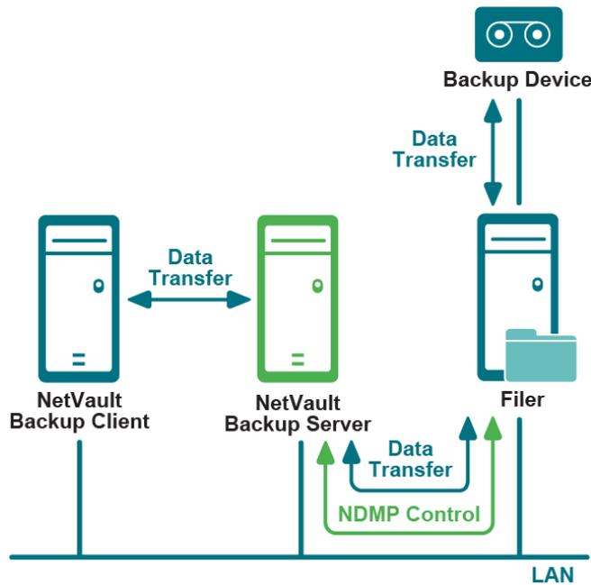
The heterogeneous three-way NDMP backup model is similar to the direct-attached model, but in this model the NetVault Backup machines on the network also use the filer-attached tape device for backups and restores.
