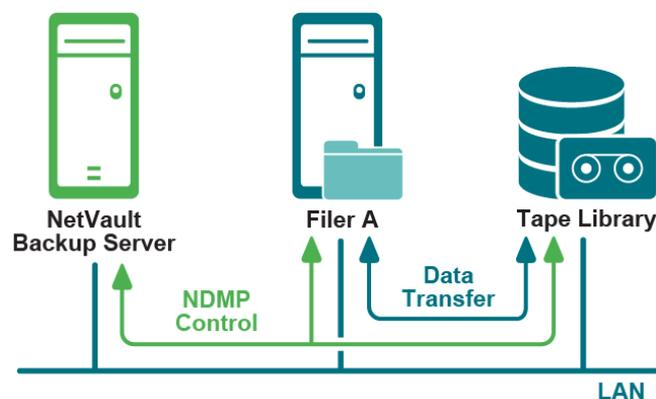
In this model, the NetVault Backup Server instructs the filer to perform backups to the NDMP-compliant network-attached storage device. The filer uses NDMP over the network to transfer the data to the storage device and backup index information to the NetVault Backup Server. The network-attached storage device can be shared by one or more filers, NetVault Backup Server and any number of NetVault Backup Clients.
