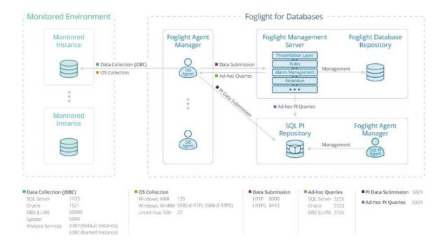
NOTE: The product components can be either distributed over different machines — preferable in large or growing environments — or centralized.
