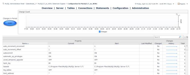
The configuration page tracks the MySQL server configuration. The metric indicator and change count graph shows numbers of changes if the selected time range. The table displays every server variable, showing the name, value at beginning and end of the selected time range, the date of the last modification since server monitoring began, and a history of changes for that variable.
