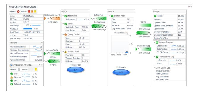
A drill-down from either the Connections or Max Connections component of the MySQL Server view takes the operator to a view of the top sessions and the SQL being executed.
