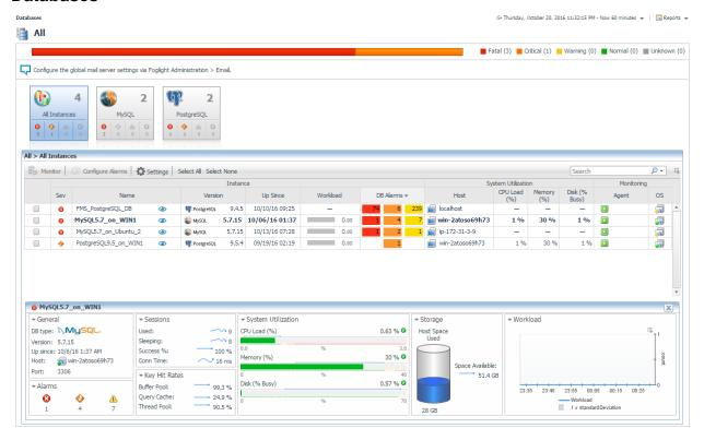
Foglight for MySQL is now incorporated into the Databases dashboard along with any other monitored database types in your environment. Like other products, the list of databases can be filtered by type and severity level and includes basic information, alarms, and host utilization metrics. Clicking on the eye icon will bring up the Quick View with more key information. Clicking the name will drill down to the MySQL Server View.
