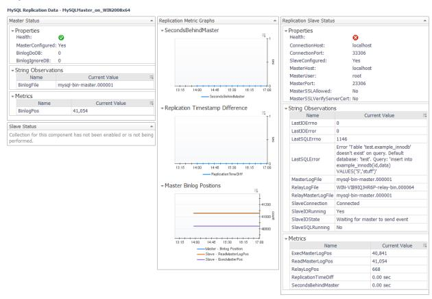
This page shows complete data on MySQL Replication collected by a single MySQL agent and will change depending on which collections have been enabled. This page is primarily meant to serve as a demonstration of data collected by the agent, but can be used for simple Master-Slave replication configurations. More complex configurations can use elements of this page in another dashboard.
