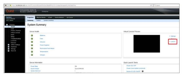
4 After the virtual console opens, log on to the system (with the username: **administrator** and password: **St0r@ge!** where the "0" in the password is the numeral zero).
