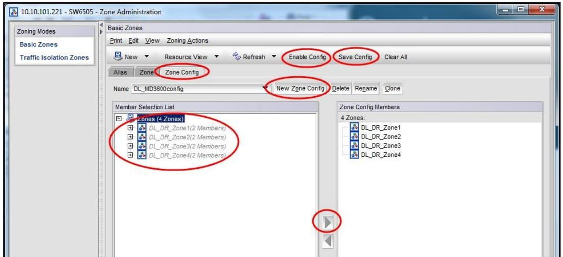
5. Repeat steps 1 - 4 to create and enable the four zones on the alternate fibre channel switch-2.
