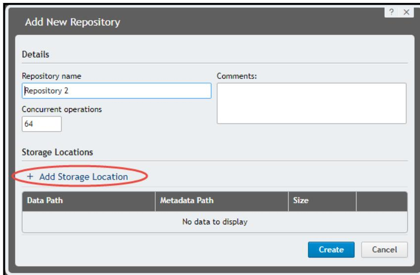
3. Select **Add file on local disk**. In this example, the DL4X00 \Data and \Metadata folders are configured to use the fibre channel storage identified by drive letter R. Select how much of the SAN LUN will be consumed by the repository (20, 40, 60 or 80TB capacities). Save the configuration.
