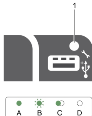
Figure 6. iDRAC Direct LED indicator
