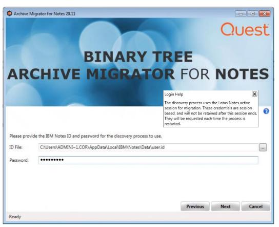
3. The user checks or unchecks the Decrypt option and clicks **Next** to continue. This screen only appears if the **Decrypt content when copied** setting is set to **User**.
