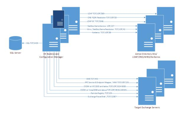
Figure 8. Ports used by File Storage Analysis collections
