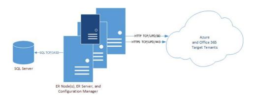
Figure 6. Ports used by Computer collections
