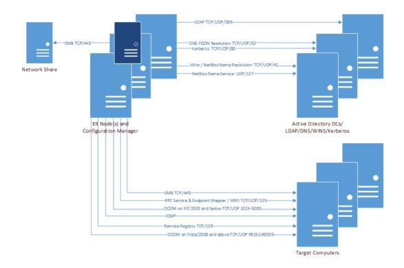
Figure 9. Ports used by NTFS collections
