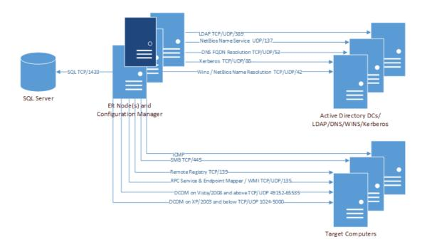
Figure 10. Ports used by Registry collections
