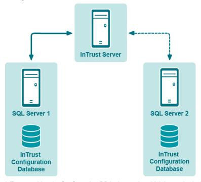
InTrust provides the Configuration DB is down rule, which is matched when the InTrust configuration database becomes unavailable to the InTrust server. This is indicated by Event ID 6565 in the InTrust Server log. The rule has the Switch Configuration DB response action, which puts a script into a temporary folder and runs it. The script switches the InTrust server to a replica of the configuration database and restarts InTrust.
