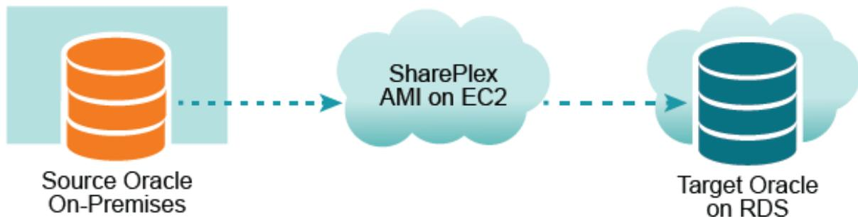
In this scenario, SharePlex runs as an Amazon Machine Image instance on the EC2 service. Capture connects to the source database through **TNS** and the Post process connects to the RDS database through **TNS**.
