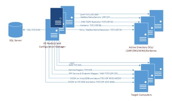
Figure 10. Ports used by Registry collections
