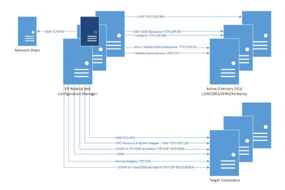
Figure 9. Ports used by NTFS collections
