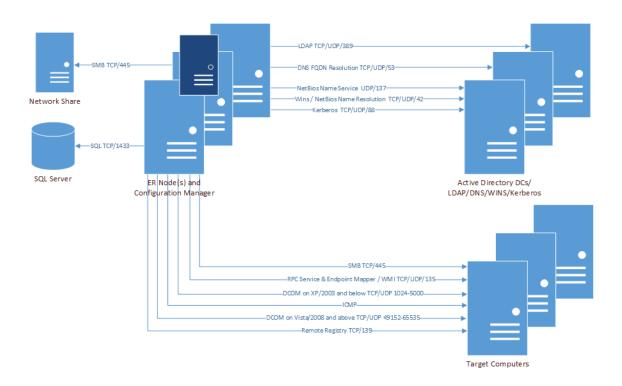
Figure 7. Ports used by Exchange collections
