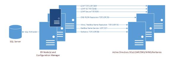
Figure 5. Ports used by Azure and Microsoft 365 collections (Exchange Online, MS Teams, OneDrive, and SharePoint Online)
