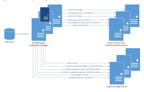
Additional port for Exchange discovery to be set on the Node:
